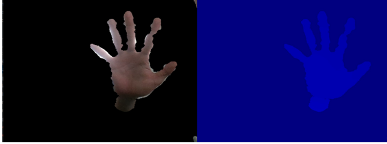
Figure 4: Hand gesture images after depth thresholding segmentation. (a) RGB image. (b) Depth image
