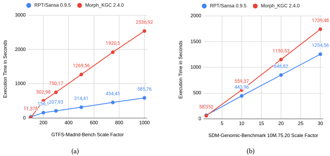
Figure 9: Execution time of RPT/SANSA and Morph_KGC with 512G RAM and all data (including temporary) in a RAM disk.
