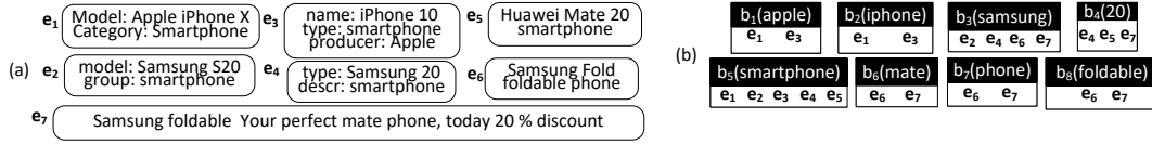
Figure 1: (a) The input entities (smartphone models), and (b) the redundancy-positive blocks produced by Token Blocking.
