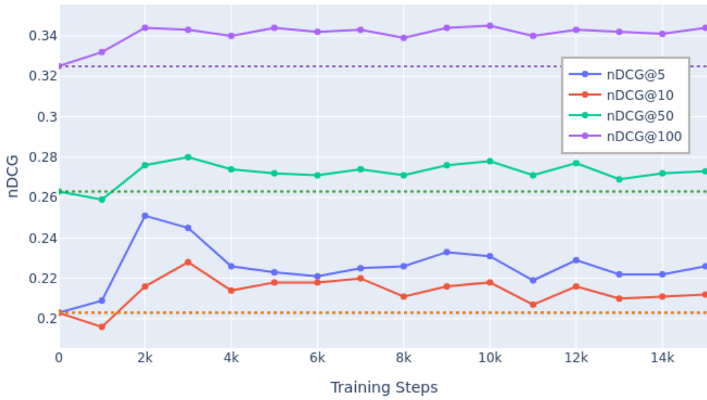
Figure 3: Performance of distilbert-base-v4 finetuned with GPL on CS data at various training steps on Top-500 Elastic Search Documents retrieved per query. Dashed lines indicate the performance of the zero-shot distilbert-base-v4 model.
