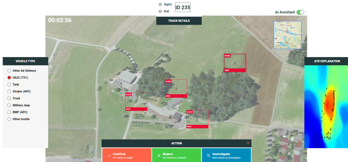
Figure 1: Screenshot of the Ethical AI Demonstrator. In the video, four objects are detected by the ATR as air defense systems. With three buttons below the video stream, the user can confirm or reject a detection or mark it for further investigation. In the list on the left, the detected vehicle type is selected. On the right, the heatmap generated by LIME is shown to explain the ATR detection.
