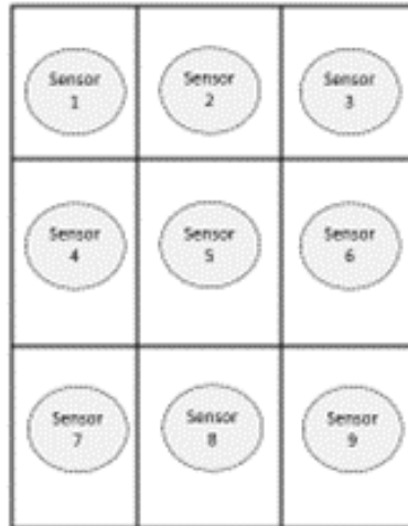
Figure 2. 3x3 sensors matrix designed to map the sheet of paper
