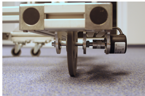
(b) Wheel-encoder installation for trolley odometry
