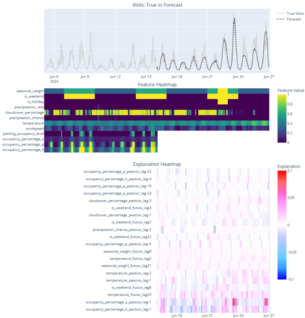
Figure 4: Interactive SHAP dashboard linking model forecasts, input features, and attributions. The shaded area indicates future covariates used during prediction. (y axis values removed for data protection reasons.)
