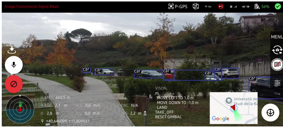
Figure 3: Execution of the TRACK command in the mobile application. The camera stream from the drone is displayed in real time, with bounding boxes highlighting only the objects corresponding to the selected “car” label.
