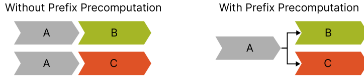
Figure 1: A visual depiction of the prefix precomputation approach for two pipelines: A \gg B and A \gg C . With prefix precomputation, the common A prefix is identified and the results are used for the computation of the remainder of both pipelines, i.e. B & C .
