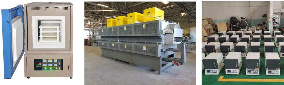
Figure 1: Examples of industrial and muffle furnaces that are actively used in production
