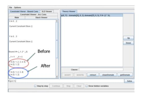
Fig. 3. PrettyCLP in action: Bounds Consistency Propagation
