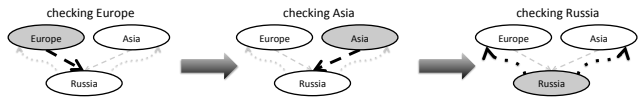
Figure 5: Step 2 for the Kaliningrad example; bold arrows highlight the edges analysed for currently handled node that is marked gray.
