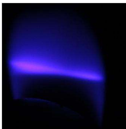
Figure 1: LII in a quasi-2-D kerosene lamp flame with 28 W 1 mm diameter cw laser beam photographed through a BG3 filter
